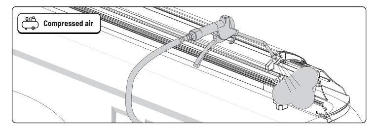
Remove dirt and debris using compressed air.
