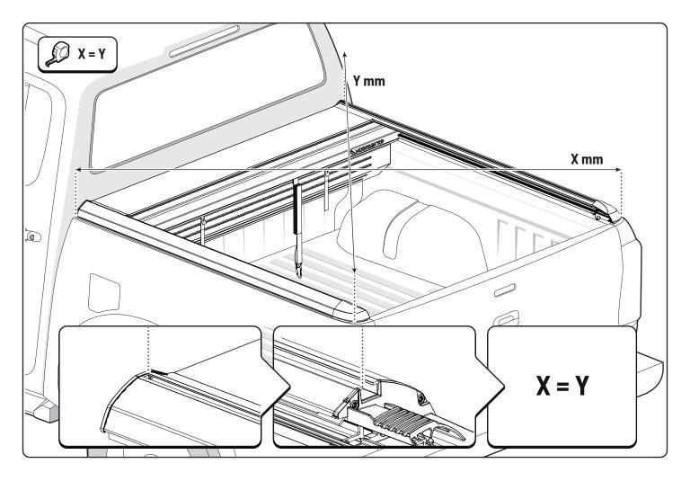
• Ensure the cross measurements are identical.
